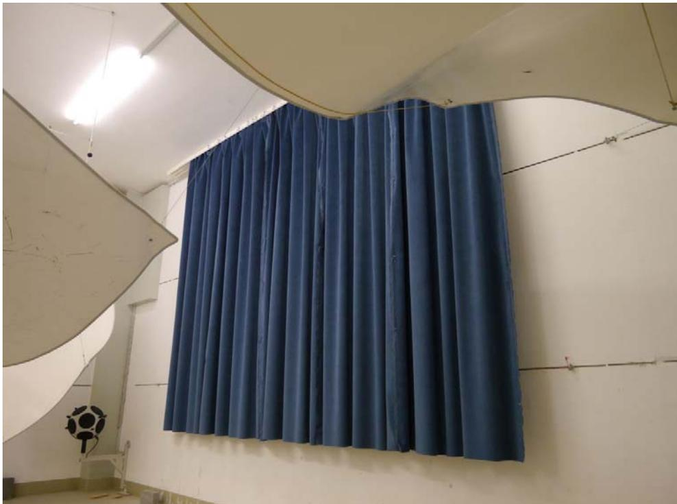
Figure B.1. Curtain arranged hanging folded with 100 % fabric addition: diagonal view.
